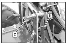
Figure 5-19: Correct forward clutch cable position.
